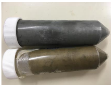
Figure 4. Subsamples of tailings from 77 m depth (grey, above) and 44 m depth (brown, below) showing the colour difference between the samples.
